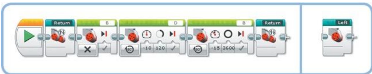
Figure 19-12. The configuration of the blocks in the Left My Block (left) and the completed My Block (right)
