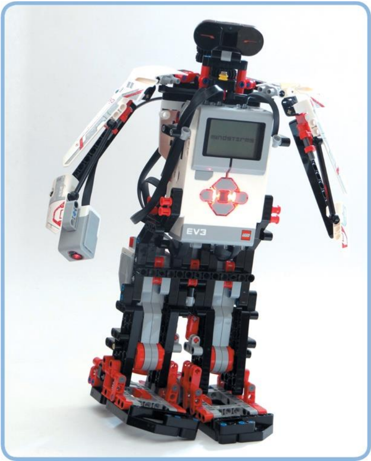
Figure 19-1. LAVA R3X walks around on two legs while moving its head and arms, and it greets you when you shake its hand.
