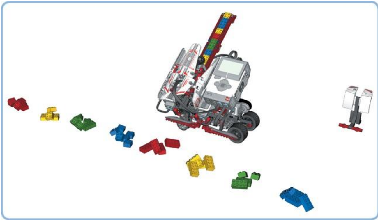
Figure 19-21. Feel like building another robot? The BRICK SORT3R sorts LEGO bricks by color (red, yellow, green, and blue) and size (2×2 and 2×4). You can find building and programming instructions at the book's companion website.
